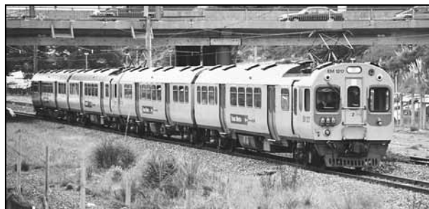
EM/ET Hungarian-built 1,500 volt dc electric multiple units. Permanently-coupled in two-car sets. Power cars (EM), trailers (ET). New 1982. Refer pages 32-33. Some preserved. Murray Jessop.
