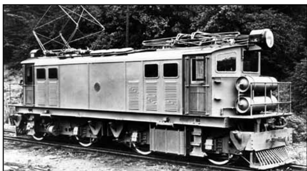
EC British-built Bo+Bo 1,500 volt dc electrics Classified E when new in 1929, reclassified EC (for electric Christchurch) in 1938, refer page 30. One preserved. English Electric photo, AC Bellamy collection.
