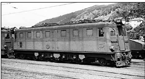
ED British & NZ-built 1-Do-2 1,500 volt dc electric locomotives. New 1938. Origin of letter D uncertain, refer page 30 for hypotheses. Two preserved. AC Bellamy collection.
