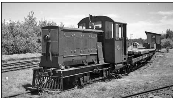
EB (2nd) NZR conversions of battery-electric EB's to diesel-electrics, starting 1953. Classification retained, although the second letter was no longer relevant, refer pages 39-40. Some preserved. Sean Millar.
