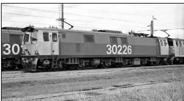
EF British-built 25,000 volt ac Bo-Bo-Bo electric locomotive. New 1988. Classification first used in public c.1991 (was previously 30). Origin of letter F uncertain, refer pages 30-31, 37, 51. In service Michael Jarka.
