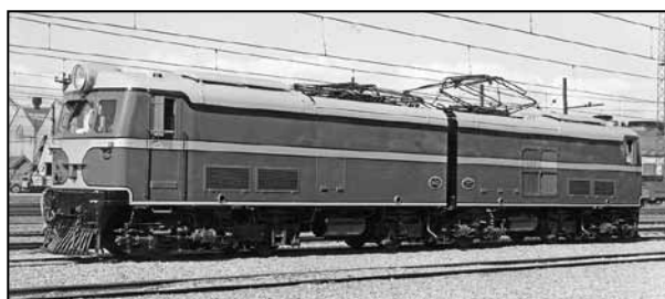
EW British-built 1,500 volt dc Bo-Bo-Bo electrics. New 1952. Classification stands for electric Wellington, refer pages 30, 66-67. Two preserved. NZR photo, AC Bellamy collection.
