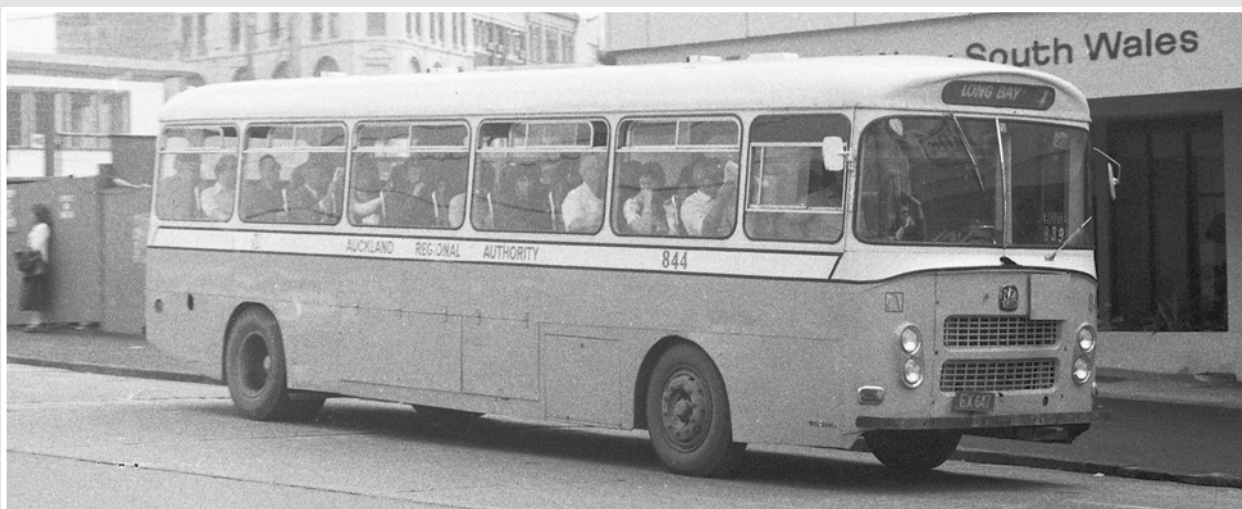
Above. No. 844 was built new with a three foot section cut from its chassis behind the rear axle, giving it a peculiar bob-tailed appearance. The standing passengers on this 1977 peak-hour service departing the central city for the North Shore, would no doubt have preferred the missing length to have been left in place! Sean Millar.
