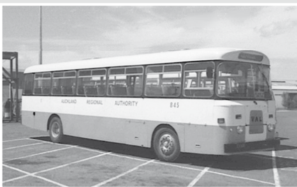
Right. No. 845 at North Shore Depot in its later years wearing the livery introduced with the MAN SL200s. By the time this photo was taken, it had been repowered with a mid-mounted Gardner engine. The remarkable conversion was undertaken at North Shore Depot. Even though the chassis no longer resembled that of a VAL, depot staff customised a VAL badge for the redesigned grille. Prior to disposal, the Gardner engine was removed, and placed in Mercedes O.305 No. 1548. No. 845’s new owners fitted it with another Gardner engine after acquisition. Paul Gourley.
