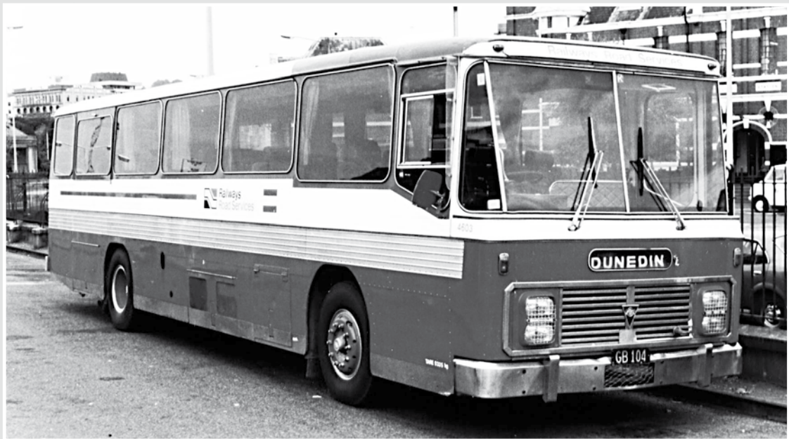
Above. No. 4603 at Dunedin in February 1981. These were the first NZRRS vehicles fitted with mid-mounted underfloor engines. Michael Jarka.
