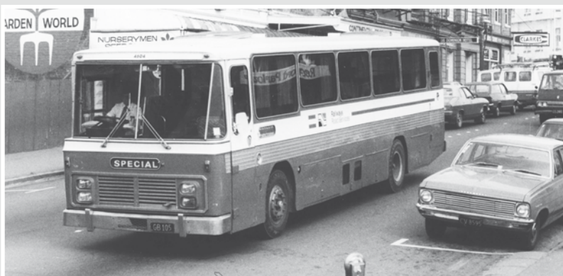
Above. No. 4603 at Dunedin in February 1981. These were the first NZRRS vehicles fitted with mid-mounted underfloor engines. Michael Jarka.
